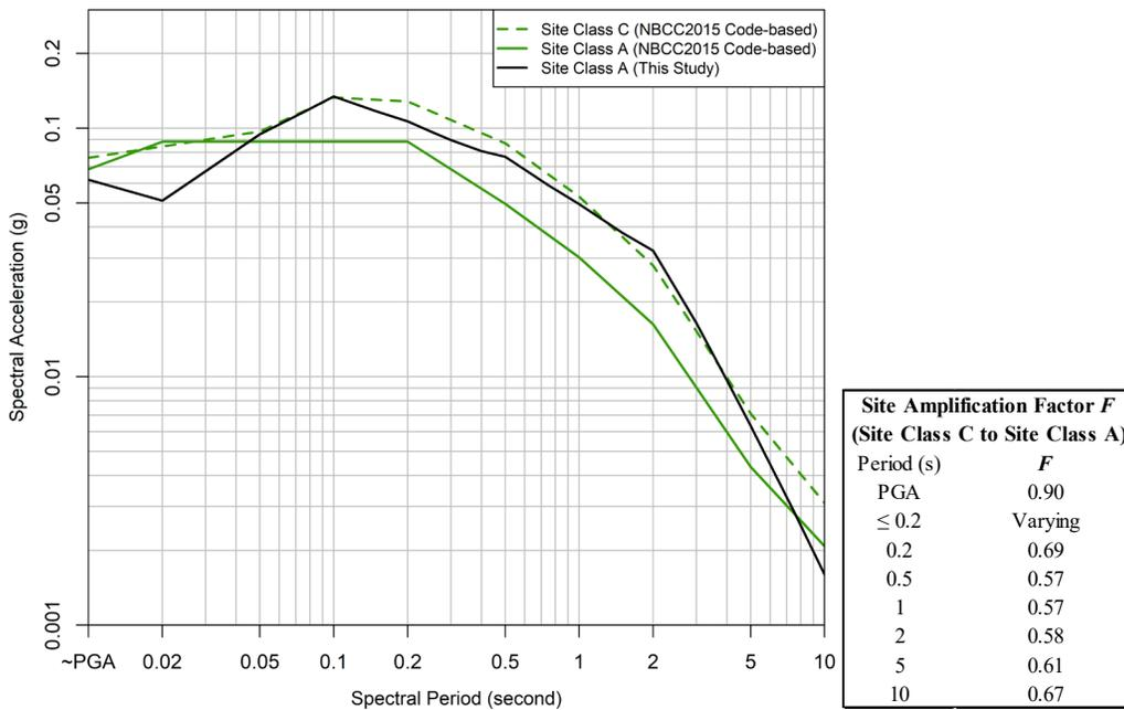
Figure 7. Comparison the UHRS (5%-damped) result to NBCC2015 code-based spectrum for an AEP of 1 in 2,475.
