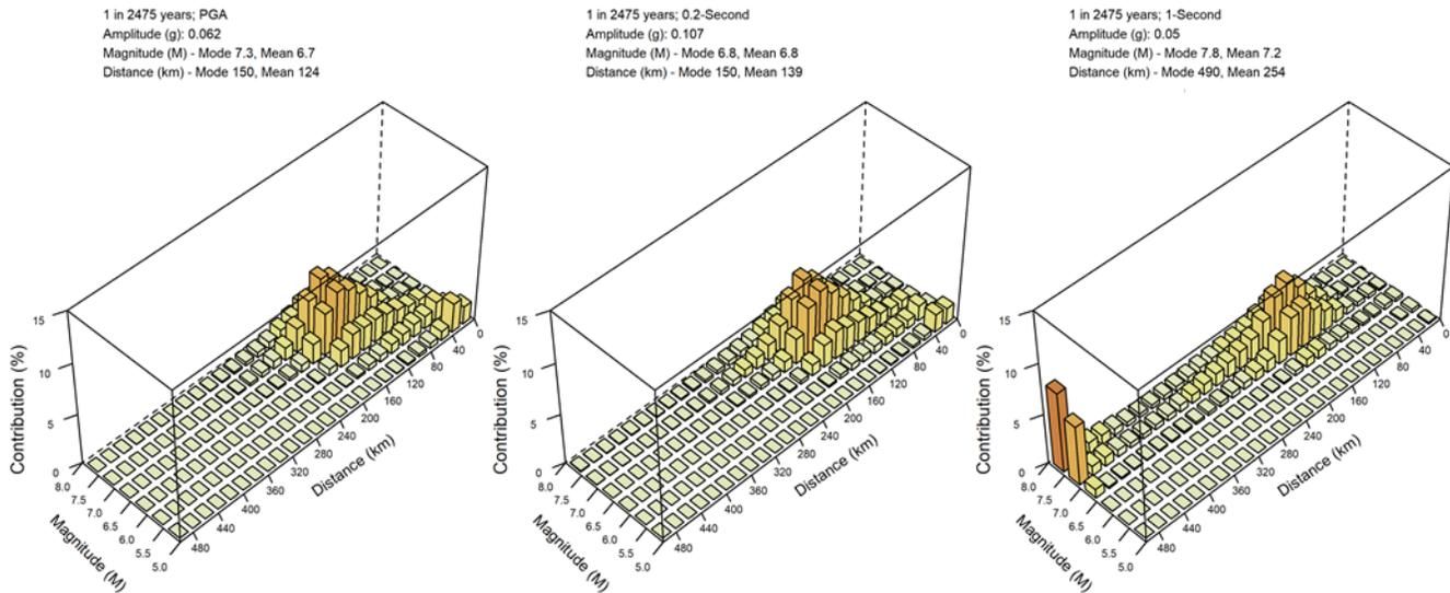
Figure 4. Magnitude-distance deaggregation for the 1 in 2,475 AEP hazard at selected spectral periods.
