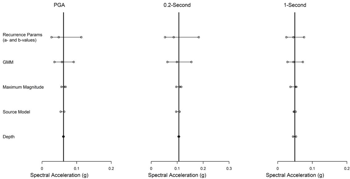
Figure 6. Tornado plots for an AEP of 1 in 2,475 at selected spectral periods.
