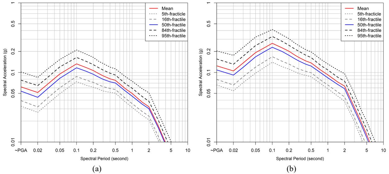
Figure 5. 5%-damped, horizontal acceleration UHRS of the mean, 5<sup>th</sup>-, 16<sup>th</sup>-, 50<sup>th</sup>-, 84<sup>th</sup>-, and 95<sup>th</sup>-fractiles for (a) 1 in 2,475 AEP, (b) 1 in 10,000 AEP.
